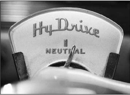
*Cars equipped with Hy-Drive wouldn't start unless the transmission was in neutral, and that's the only position marked on the selector quadrant.*
